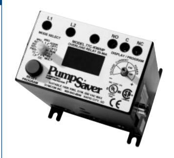
The Model 77C-KW/HP has important advantages over current monitors in many protection applications. Any motor load that has a small or very non-linear change in current vs. load requires the use of a power monitor for underload, dry run and dead-head protection. The change in power vs. load is more linear for most motor loads and is greater in magnitude than the change in current in all motor loads. This is because power measurements take into account both power factor (pf) and current.
